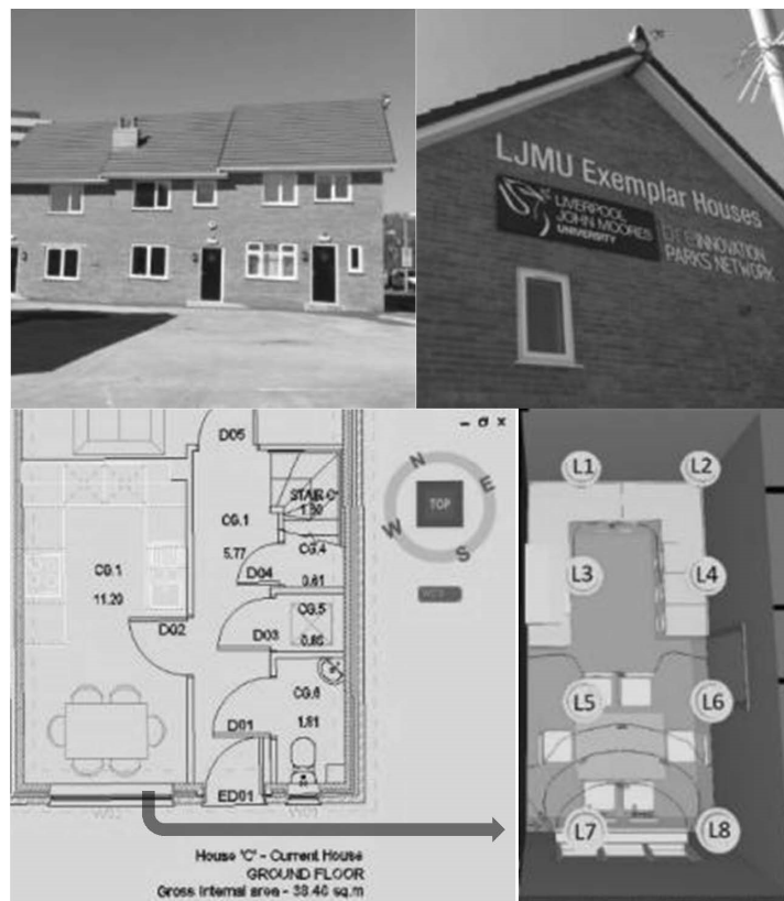
Figure A1. Liverpool John Moores University (LJMU) Exemplar houses ( top ). The Computer-aided Design (CAD) drawing and lighting DIALux model ( bottom ).
