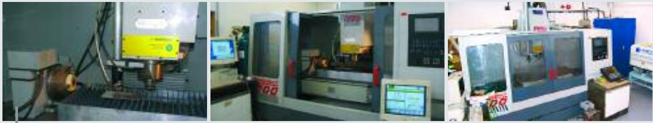
Trumpf TLF1200W laser. The beam is enclosed within tubes but bounces off a series of mirrors into a 4 axis Bridgeport CNC machining center
