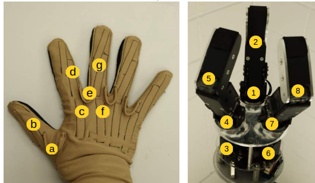
Figure 4.4: Joint mapping scheme between the Cyberglove and the custom robotic hand.
