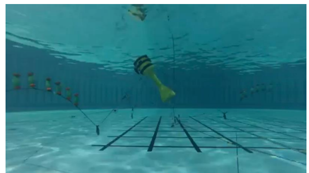
Fig. 5. Survivability testing of a 1:40 OWC spar buoy model in the FloWave tank.
