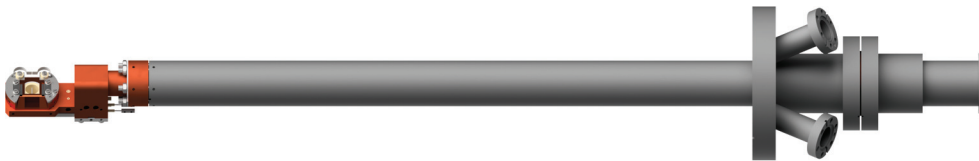
Figure 4.4: Rendered image of the preparation chamber manipulator head attached to the cooling finger and the CF63 cluster flange. The whole part is mounted to the manipulator, which is equipped with a rotational feedthrough.
