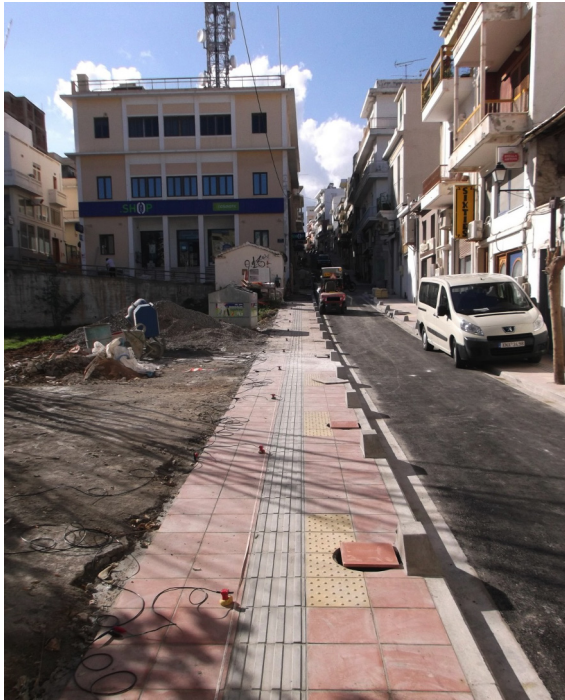
Figure 4. Receiver array set-up for MASW and linear MAM surveys at station AGNA. Geophone spacing of 3 m is shown.
