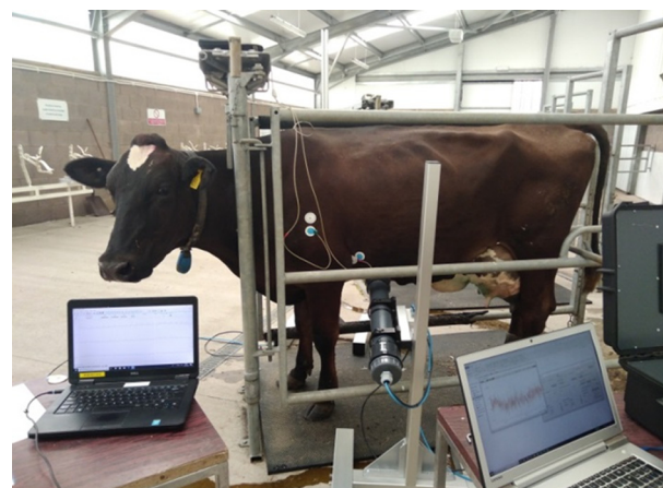
Fig. 1. Non-contact heart recording: Two magnetometers were placed either side of the animal so that an imaginary axis passed through the heart muscle. Simultaneously an ECG was recorded. One magnetic sensor can be seen in front of the animal placed slightly back of the fore leg and below the heart.
