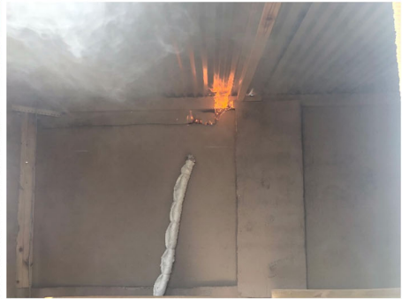
(b) Cardboard lining ignition of ISD2
