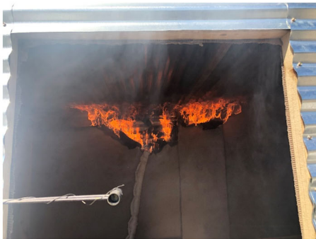
(c) Spread across the cardboard lining of ISD2
