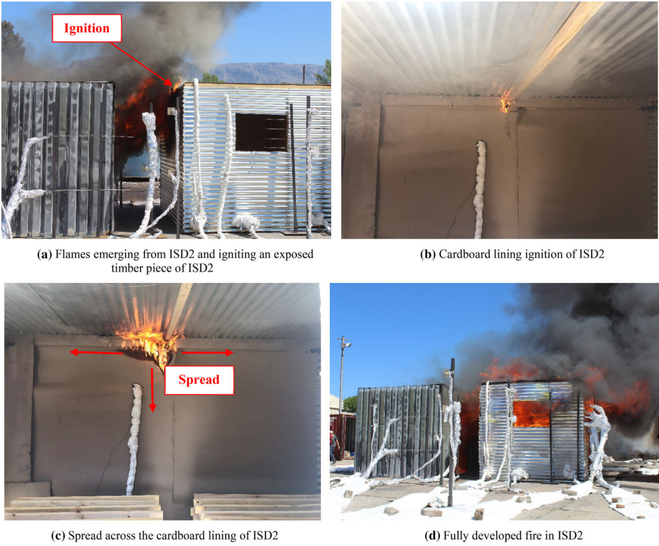
Figure 8. a Flames emerging from ISD2 and igniting an exposed timber piece of ISD2, b Cardboard lining ignition of ISD2, c Spread across the cardboard lining of ISD2, d Fully developed fire in ISD2.
