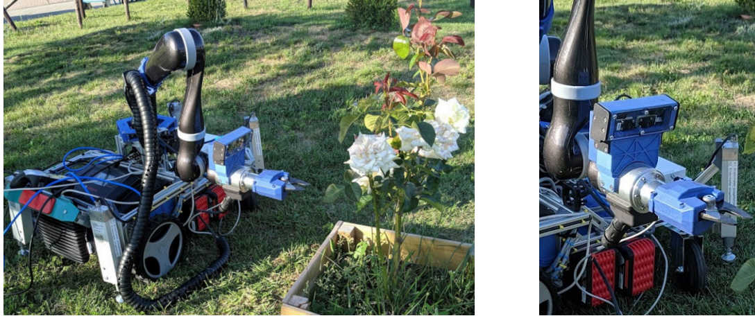
Figure 1: General overview of the robot (left image) including the 6-DOF robotic arm and the cutting tool. A stereo camera using an eye-in-hand configuration (right image) is mounted on the same cutting tool.
