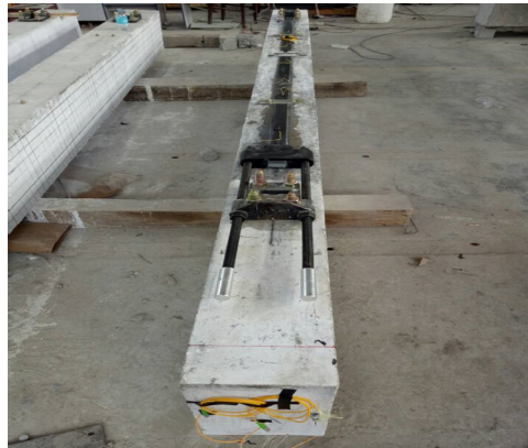
Figure 9. An RC beam specimen after installation of the prestressed SCFR plate.
