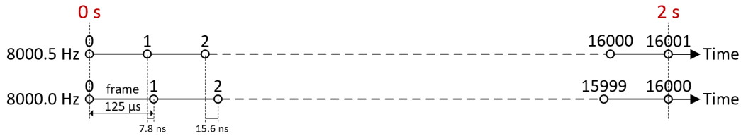
Fig. 3. Explanation of clock drift.
