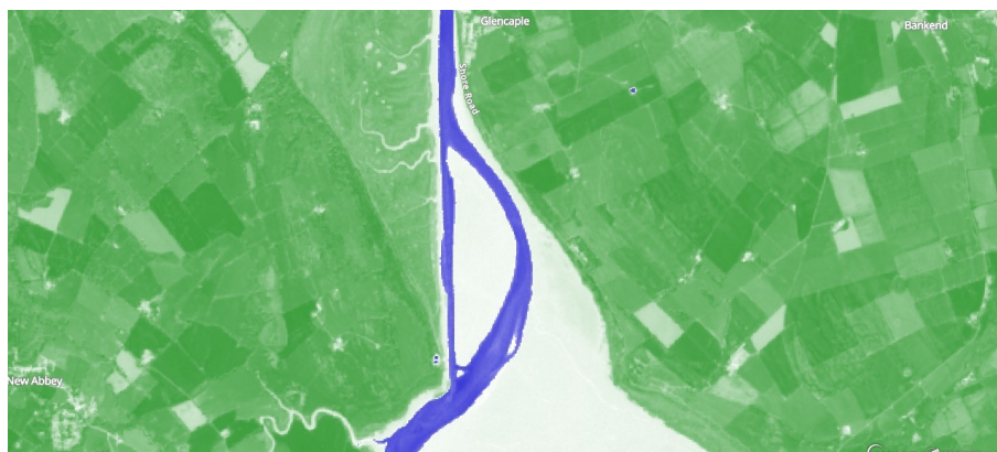
Figure 2: NDWI image of the Solway Firth at low tide processed from Sentinel-2 data. Blue shows location of water channels.
