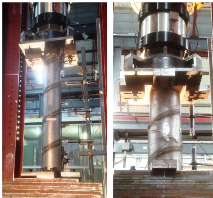
Fig. 8 – Spiral welded composite columns, Aslani et al. (2017)
