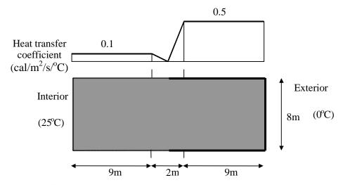
Figure 10 Geometry and boundary conditions, concrete column problem
