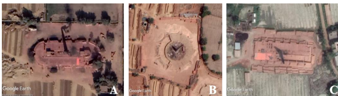
Figure 4.2: Examples of the three dominant types of kilns which are found across the ‘Brick Belt’. All images were captured by WorldView satellites – DigitalGlobe/Maxar Technologies – and downloaded from Google Earth Pro (23.05.2020). A: captures a BTK which is found near Lahore, Pakistan (31 54 27.55 N, 74 13 32.88 E) and was captured during the brick-making season on 06.12.2017, hence the smoke which is visible from the centralised chimney. B: is a circular kiln found in a kiln cluster near Jaipur, India (26 54 6.23 N 75 57 14.97 E); captured 08.04.2020. Finally, C: is a Zig-Zag kiln – notable due to the rectangular shape. This kiln was captured on 25.04.2018 in a large cluster of kilns to the north of Dhaka, Bangladesh (24 1 12.01 N 90 20 27.69 E).
