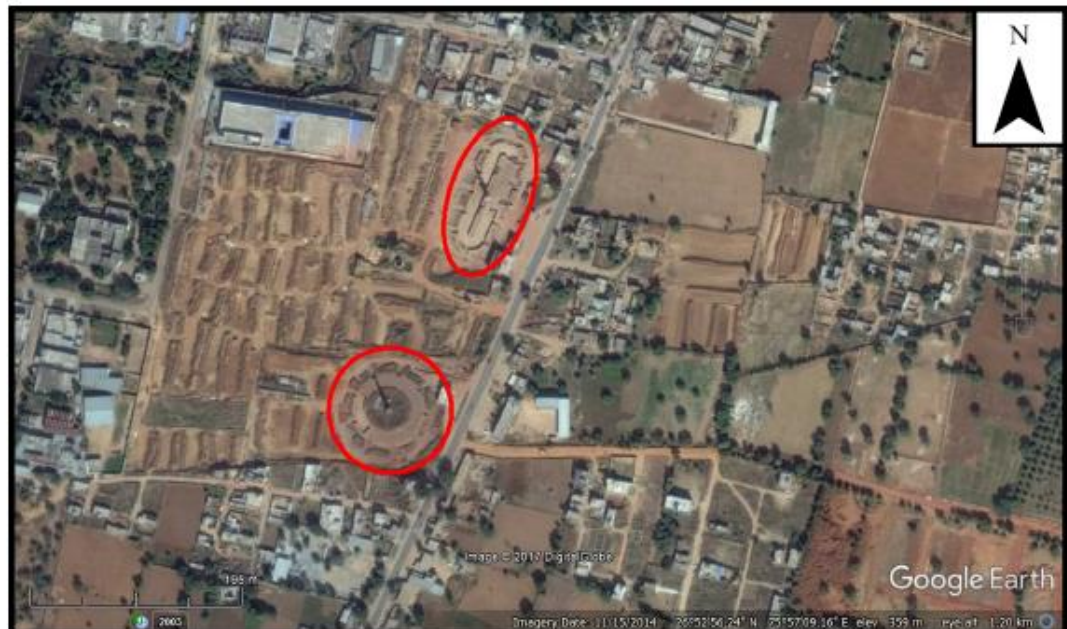
Fig. 2. An image featuring two brick kilns. One is a traditional Bull's Trench Kiln (BTK) and the other is a circular kiln. Surrounding these kilns is a number of clay fields that are used in the production of the bricks themselves before the firing of the bricks in the kilns. These fields are commonly found close to the kilns although sometimes they are not directly adjacent to the kilns.
