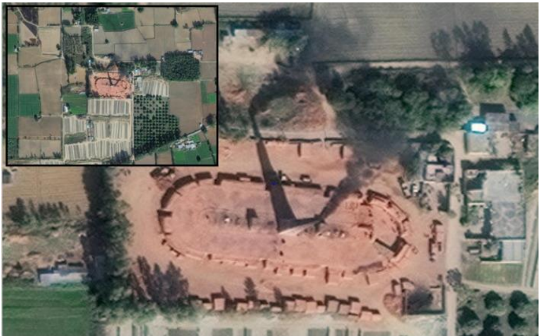
Figure 4.7: An example of a Fixed Chimney Bull's Trench Kiln (FCBTK) at 31 32 18.798 N, 75 58 52.975 E – note the emissions from the chimney stack. Image from DigitalGlobe's WorldView-2 satellite system; pan-sharpened natural colour at 50 cm spatial-resolution; captured in November 2015.
