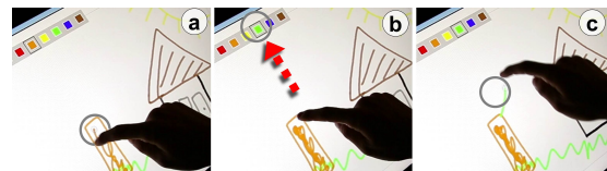
Figure 8: Remote-Colour-Select: a user draws the tree stem directly (a). The user then changes to the ‘green’ colour by a look at the corresponding menu icon, and a tap (b). The user directly continues drawing (c).
