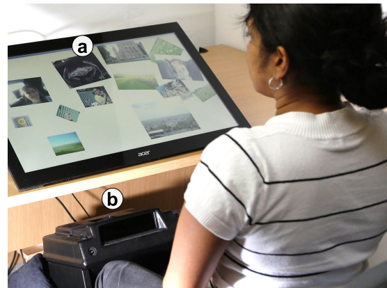
Figure 7: The system consists of a 27" 1080p multi-touch sensitive surface (a), and the 120hz Eye Follower eye tracking device (b).
