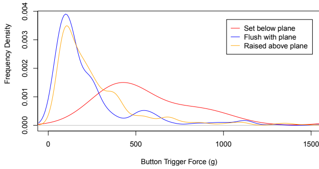
Figure 1. Peak force required to trigger buttons, based on relationship to surrounding plane
