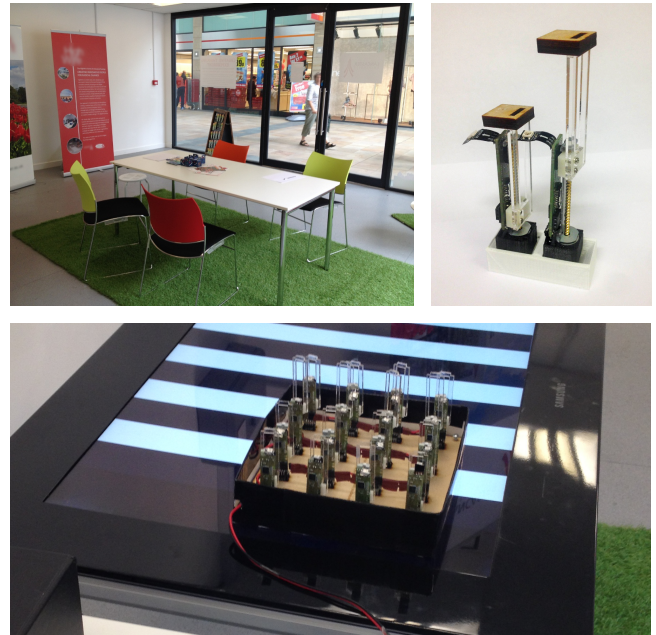
Figure 1. (Top left) Study location; (Top right) ShapeClip display components (minimum/maximum heights); (Bottom) Public demonstration using 16 ShapeClips [14].
