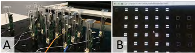
Figure 7: Actuators in specific positions on an 8x6 grid above flat monitor (A); Height control webpage underneath (B).
