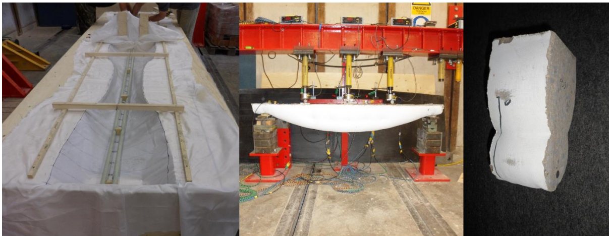
Figure 1 Flexibly-formed beam cast in hung from fixed edge supports
