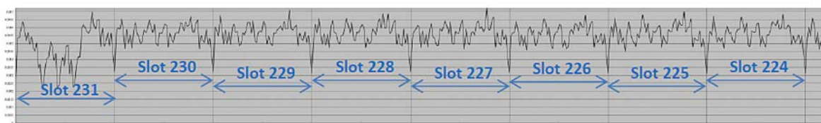
Fig. 1. First 8 slots of the simulated Power Trace for the case 1: the IHP kP -design processed the EC point P_I=(x_I, y_I) as the input data using the scalar k_I .
