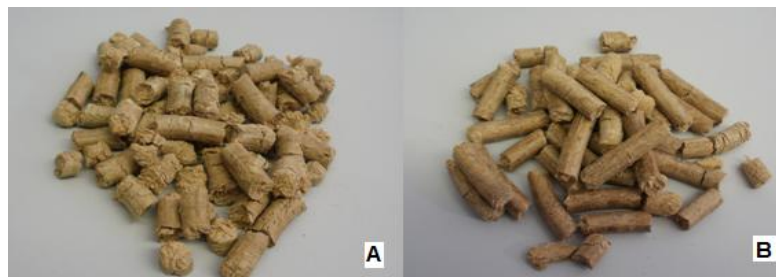
Figure 4.11: Pellets from rice husks, applying less force (A) and more force (B)
