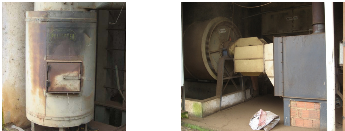
Figure 5.4: Coffee husk furnace (on the left) for drying coffee beans (on the right)
