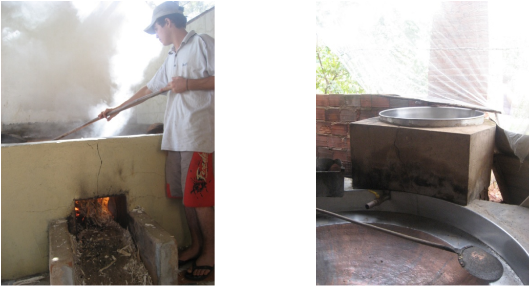
Figure 6.2: Formal pan for juice cooking (left) and new “double pan” (right).
