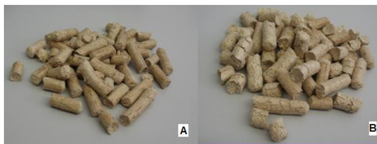
Figure 4.12: Pellets from sugar cane bagasse grinded to 2 mm (A) and 4 mm (B)
