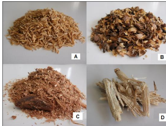
Figure 4.4: Raw biomass: rice husks (A); coffee husks (B); Eucalyptus saw wood (C); sugar cane bagasse (D)
