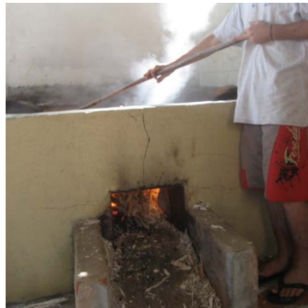
Figure 5.8: Sugar cane bagasse (on the left) and bagasse combustion for cooking sugar cane juice (own source)
