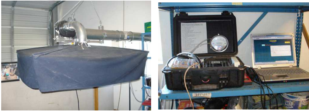
Figure 48: The emission collection hood, sampling system and computer
