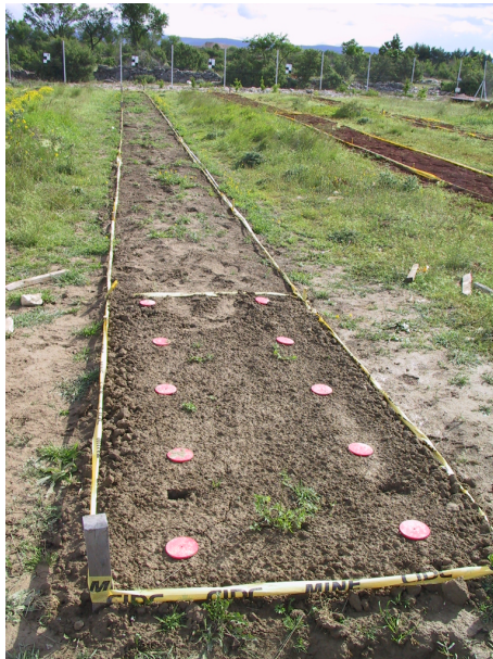
Figure 7.3: Area fully prepared for the maximum detection height measurements. The target positions and their depths are clearly indicated with red markers.
