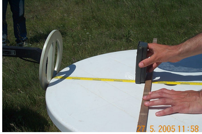
Figure 7.4: In-air maximum detection height measurements. The target is being moved, while the search head is kept still.
