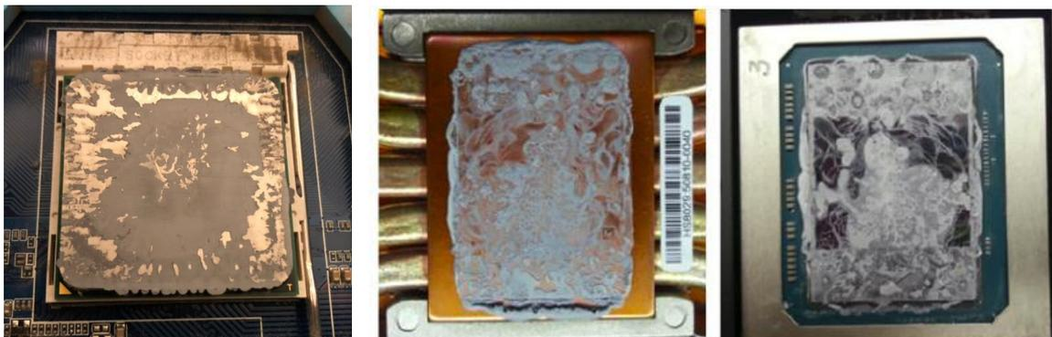
**Figure 4.37:** Examples for degradation of thermal contact
