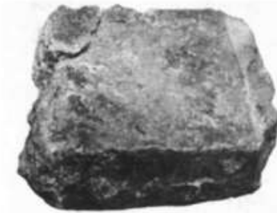
PLATE 9.3 Glass frit block showing the flat upper surface, lateral sides and a part of the fritting crucible left adhering to the right side
