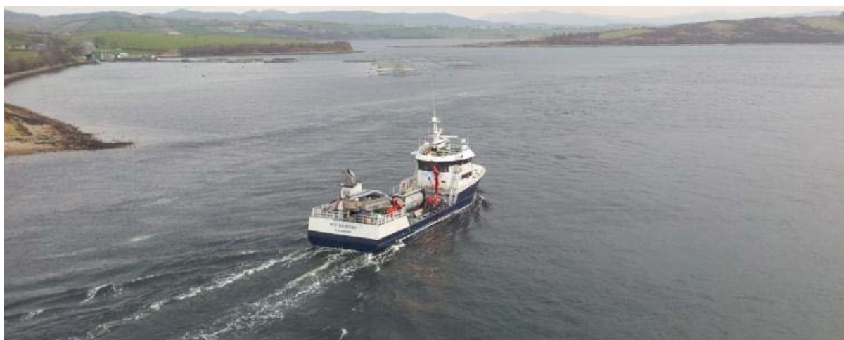
Figure 1. Specialised transport wellboat for moving salmon between sites. Such movements require approval by the CA office in the Marine Institute and strict biosecurity measures are applied to prevent potential spread of aquatic pathogens.
