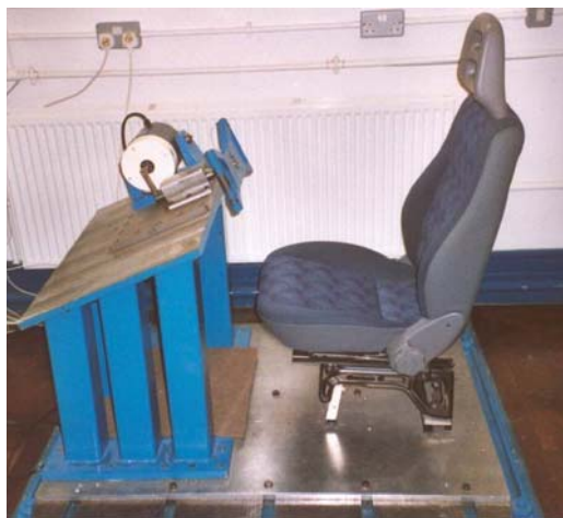
Figure 1) Steering wheel rotational vibration test rig.
