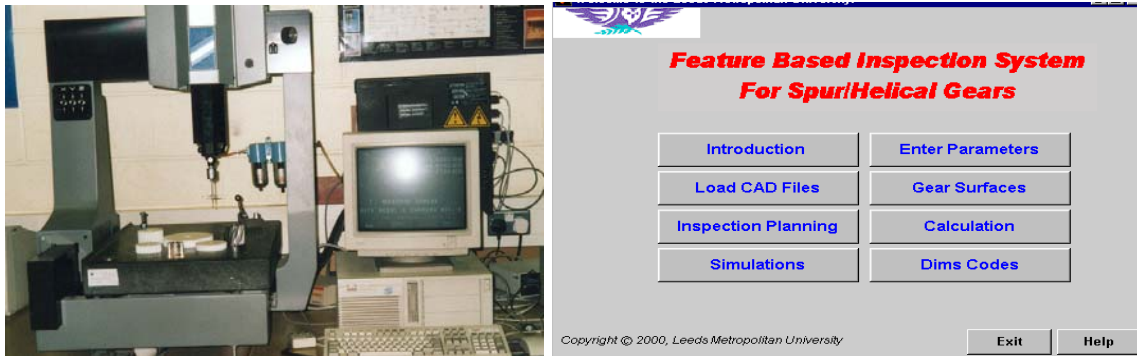
Fig. 7. Measurement system and Interface of the developed inspection system
