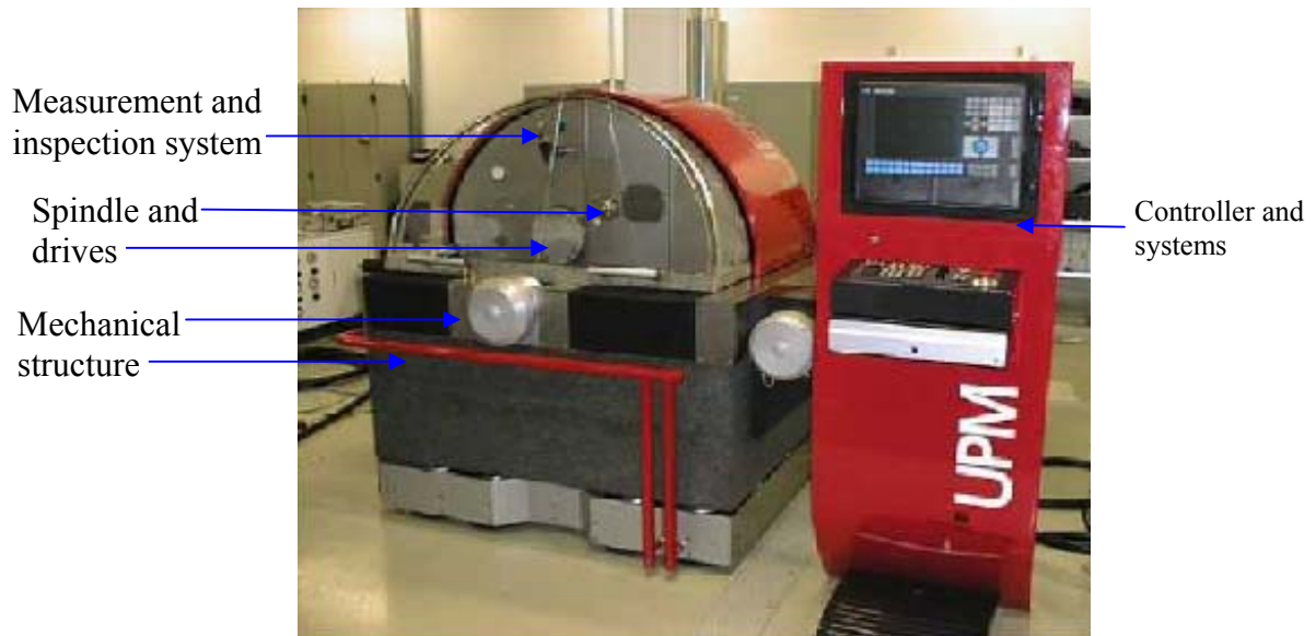
Fig.1 Schematic figure of an ultraprecision milling machine [3].
