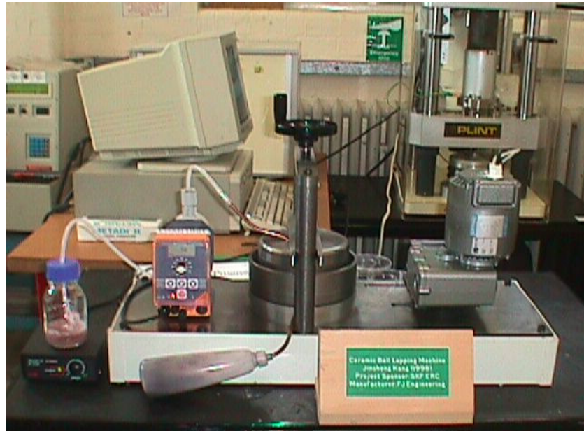
Fig. 1 Overview photograph of the eccentric lapping machine
