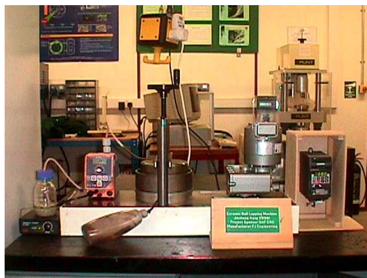
Fig. 6 Overview of the novel eccentric lapping machine
