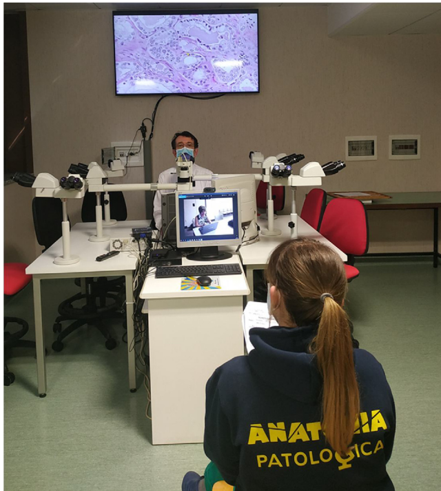
Fig. 1 – A pathologist uses a multiple-head microscope with a digital camera and a TV screen showing an image of prostate cancer. The equipment is associated with a computer and a monitor showing a remote participant discussing the case. The audience is composed of a resident sitting at a distance from the microscope.
