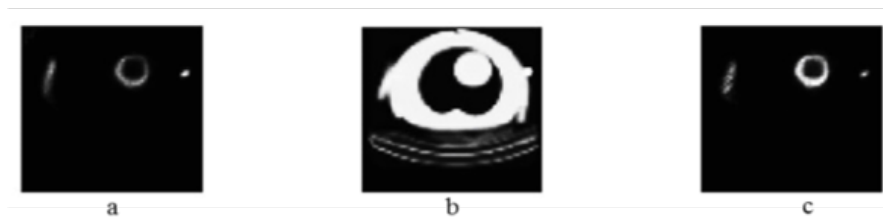
Figure 10. OSEM reconstructed image. Before attenuation correction (a) attenuation map (b) after attenuation correction (c).
