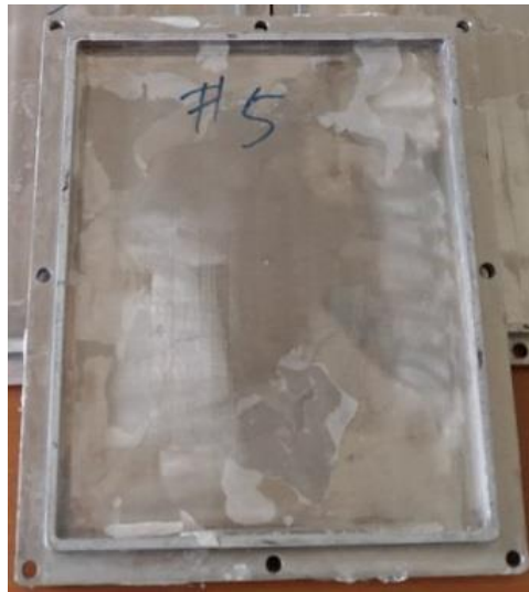
Figure 4. Mold for CIPP sample production.
