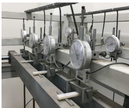
Figure 6. Creep test loading.
