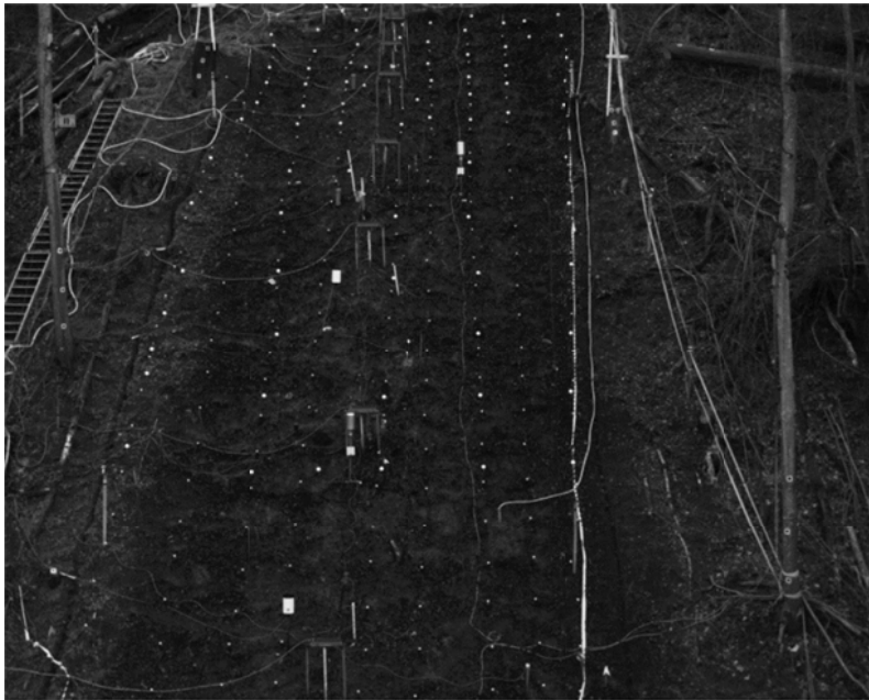
FIG. 9. An image taken from CAM3 in the evening at 6:00:00 pm. The smaller white spots are the ping-pong balls of the first experiment. The larger white ones are the tennis balls.
