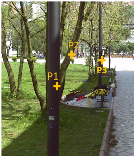
Figure 11. Test objects and selected points P1-P3 for error ellipsoid plotting. P1 and P3 selected from lamp poles, and P2 from branch of tree
