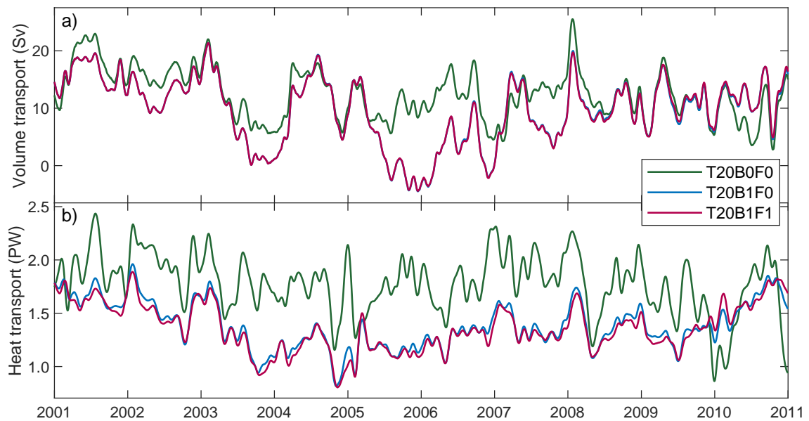
Figure 4.19: Meridional volume (a), and heat (b) transport through the Atlantic Ocean at 26.5^{\circ}\text{N} calculated from three MPIOM model experiments, smoothed with a Gaussian-weighted moving average filter with 60 days window length.
