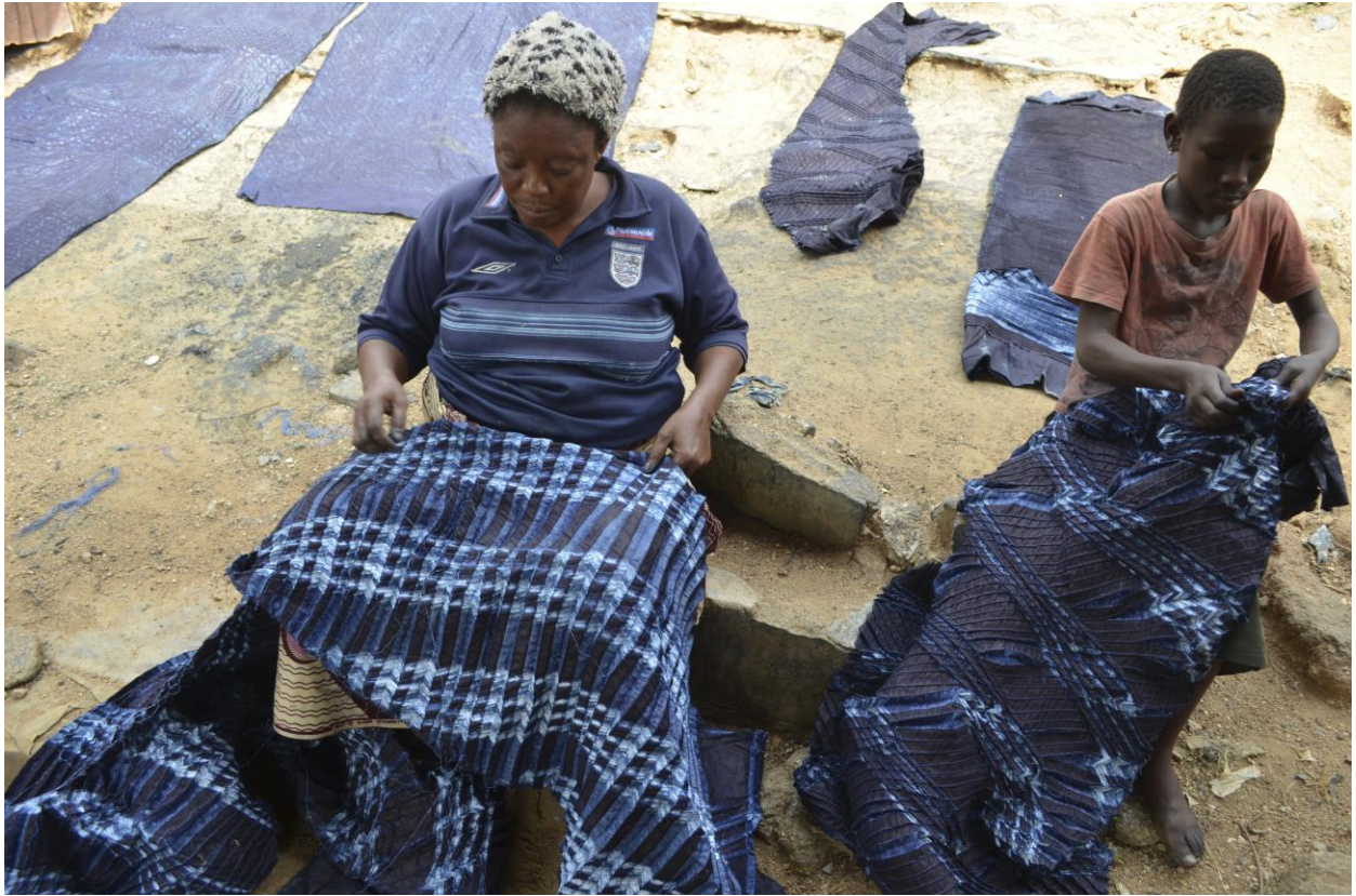
Figure 3.9 Removing the thread from a sewn-patterned adire at the Ijemo factory, Abeokuta March 2014. Photo by the author.
