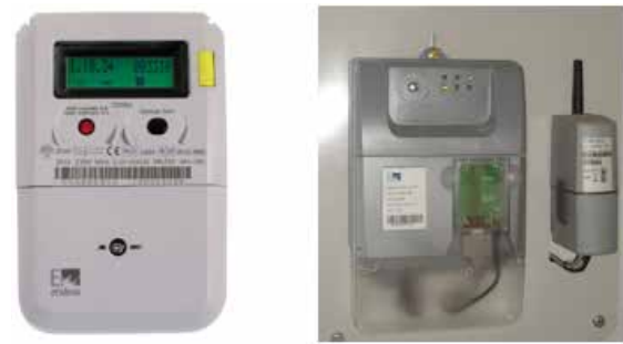
Fig. 24. Smart meter and concentrator installed in Smartcity Málaga (courtesy of Endesa).
