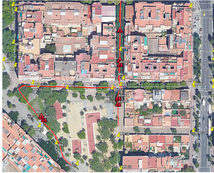
Fig. 9. Inspection report of the experiments at Virrei Amat square. The path followed by the SIAR platform is marked in a red line. The generated alerts by the system are shown in red exclamation marks.
