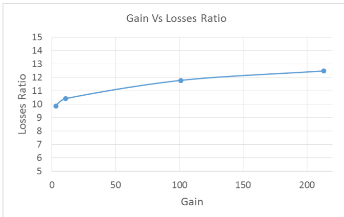
Figure 4.42 System losses ratio depending on the amplifier gain.
