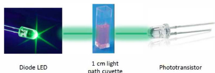
Fig. 2. Schematic system of the optoelectronic system detection.
