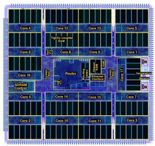
Fig. 1: SpiNNaker chip layout [1]. It contains 18 ARM processors, a Router and SDRAM controller.
