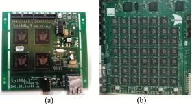
Fig. 2: (a) 4 chip SpiNNaker board [SPIN-3], (b) 48 chip SpiNNaker board [SPIN-5]
