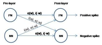
Fig. 4: Pre-layer post-layer connection scheme. e(w) is excitatory target and i(w) is inhibitory target
