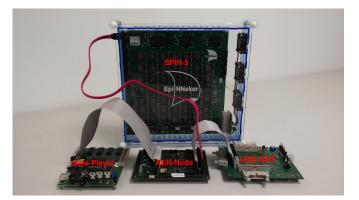
Fig. 5: Experimental setup. Events flew from Data-Player [11] to AER-NODE board [13] to SPIN-5 board. The processed events come back from the SPIN-5 board to AER-NODE board and they go to USB-AER [11] board to be sent to the computer.
