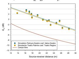
Figure 12. Variation of the spectral simulated value of  $G_m$  (average of 0.5 and 1 kHz) against source-receiver distance.
