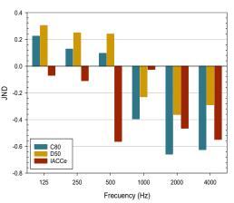
**Figure 11.** Spectral behaviour of the differences between the spatial averages of simulated values of the acoustic parameters:  $C_{80}$ ,  $D_{50}$ , and IACC<sub>E</sub>.
