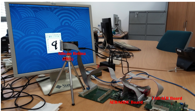
Fig. 3: Hardware setup for real-time processing with DVS. A video of the real-time demonstration is available in [22].
