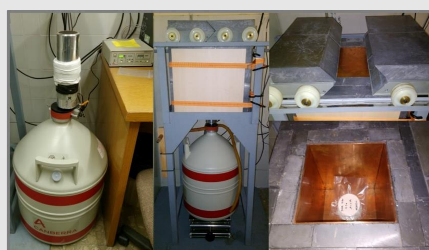
Gamma-ray spectrometry system used in this study: HPGe detector and lead shielding.
