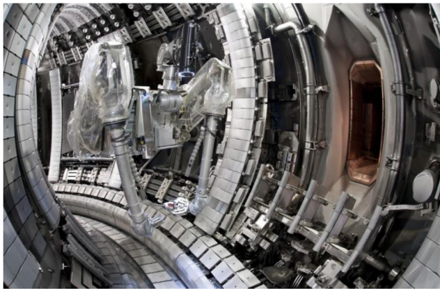
Figure 2. Left: remote Handling MASCOT inside the JET vacuum vessel. Right: the neutron generator deployed by the MASCOT and the power supply control unit (PSCU) attached to the MASCOT body.
