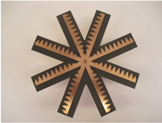
Fig. 12. Top photographic view of the manufactured prototype of the radial array with N = 8 sinusoidally modulated HMLWAs.
