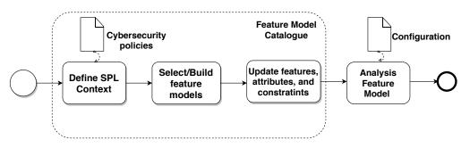
Figure 4. Process for verifying compliance of cybersecurity policies.
