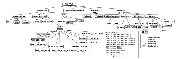
Figure 10. SSL/TLS Feature Model.
