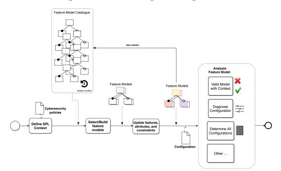
Figure 5. CyberSPL workflow with feature model catalogue.
