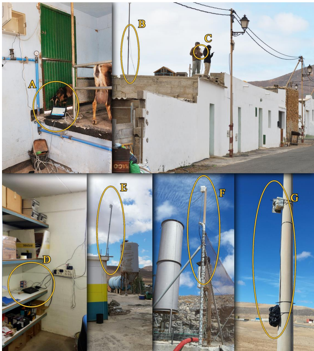
Figure 6. Details of the required system for the correct functioning of UvABiTS devices. (A) Laptop installed close to the main supplementary feeding station conforming the base station number 1. (B) Antenna connected to the laptop 1. (C) Relay used during the installation of a supporting relay for base station 1. (D) Laptop installed close to the garbage dump conforming the base station number 2. (E) Antenna connected to the laptop 2. (F) Relay installed inside the garbage dump supporting the base station 2. (G) Another relay installed inside the garbage dump supporting the base station 2.
