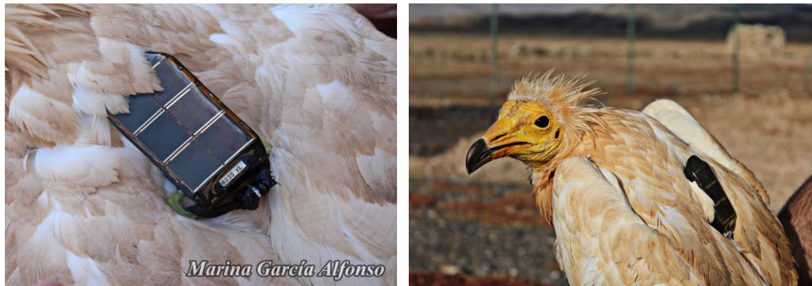
Figure 4. Details of an UvABiTS device on the left and a Canary Egyptian vulture equipped with an UvABiTS device on the right.
